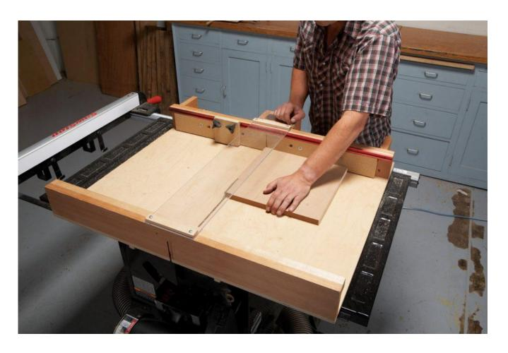
On a crosscut sled, the fence must be absolutely square to the blade. Here's a super-accurate method of testing for square. It makes errors easier to detect by magnifying them by a factor of four. The same method also works for a miter gauge, using smaller test pieces.
