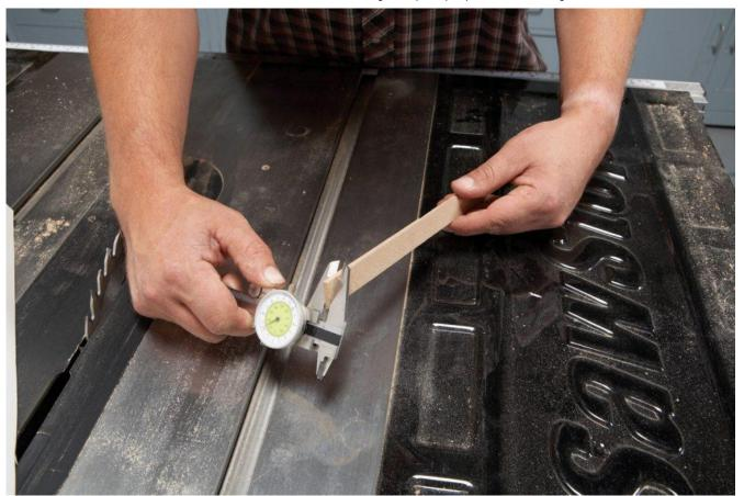
Use a caliper to precisely gauge the sliver's thickness. If your fence is perfectly square, this sliver will be the same thickness over its entire length. If your fence is not square, the sliver will be thicker at one end than the other. The difference in thickness indicates four times the amount of error in each cut. Keep adjusting the fence by minute amounts, repeating the procedure until the last sliver is perfect. –Joe Emenaker
